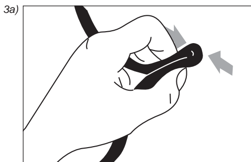
Fig. 3a + 3b Strain relief for flat actuator wires.
