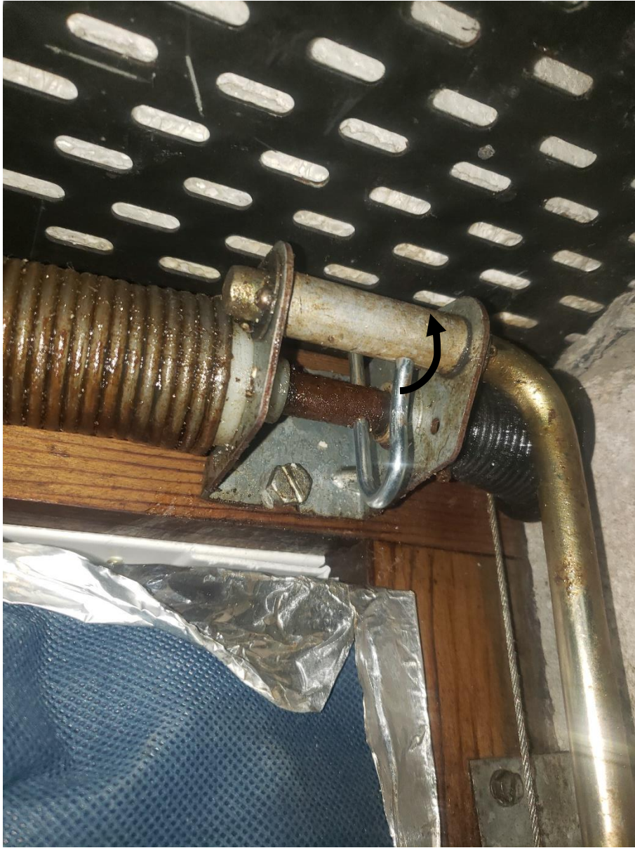
Figure 2-new position of crook pin (over the tube, as shown by black arrow)
