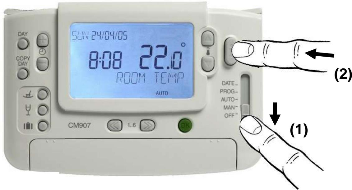
1. Move the slider switch in the OFF position
