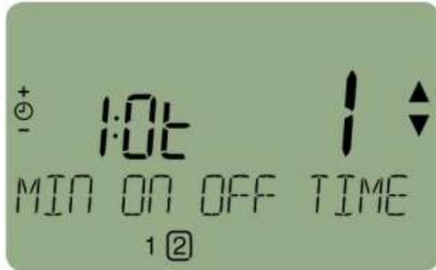
1. To enter the second level of parameters press the PROG >> key (period)
