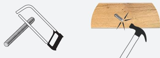
Insert the threaded rods into the holes in the beam, drive all the way in with a hammer. Cut down the threaded rods with a hack saw if necessary.
