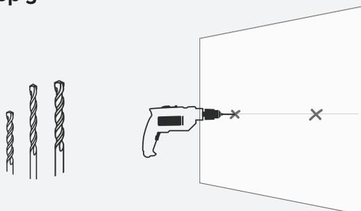
Drill to a depth of **75mm** using first a **7mm** drill bit then a **12/13mm** drill bit and finish with a **18mm** drill bit.
