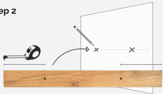
Drill required number of holes in the middle of the beam to a depth of 125mm with a 16mm drill bit. Measure from the end of the beam, to the centre of the holes and transfer these measurements to the wall.
