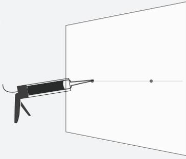
Inject mortar resin into the back of each drilled hole until around half full.
