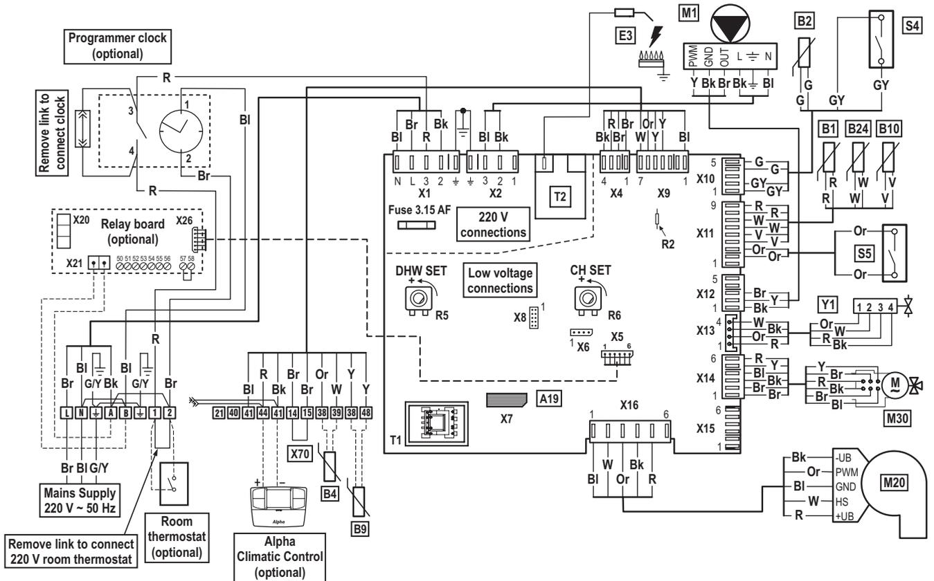
When an Alpha Climatic control is connected to terminals 41 and 44 remove the links between terminal blocks 1 and 2
