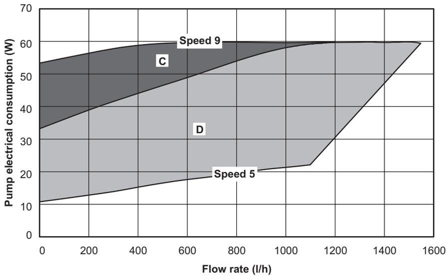
C + D = Pump power consumption with by-pass opened.
