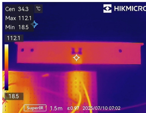
Expt1: glued-on with Thermal Glue*
