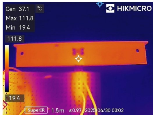
Control: bolted-on with heatsink compo.
