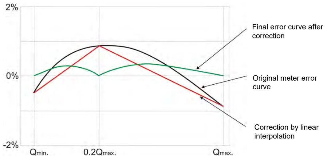
The initial error curve of the diaphragm gas-meter is introduced into the micro-processor in the index at 3 flows,  $Q_{min}$ ,  $0,2 Q_{max}$  and  $Q_{max}$ . With the High Frequency “Gray-Code” detection, flow is calculated and by linear interpolation and the error curve of measuring unit corrected to approx. 0.1%.
